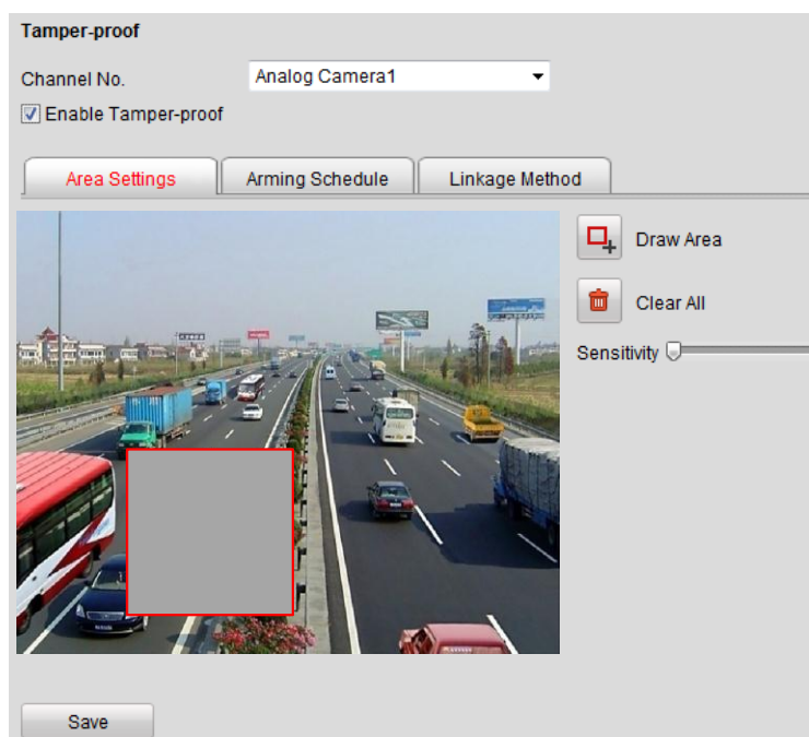
Figure 8.22 Tamper-proof Alarm Settings
